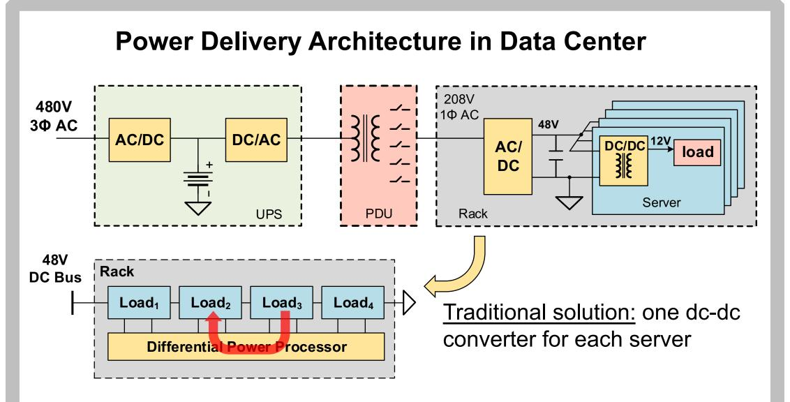
A 50V to 5V solution with 10 series-stacked voltage domains:
