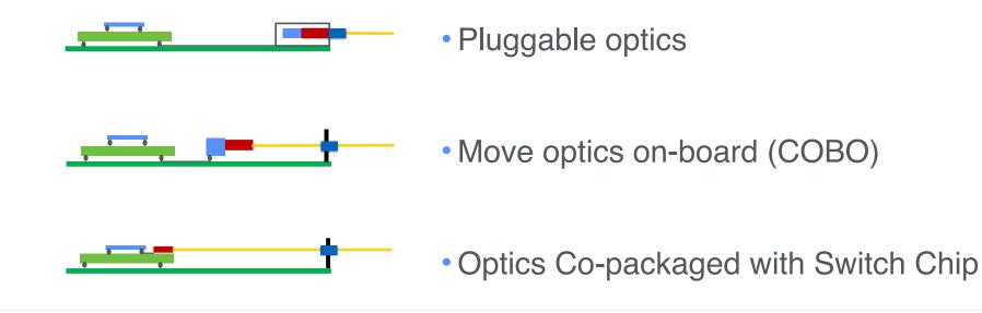
Co-packaged optics enable much lower-power electrical I/O with a potential 30% power reduction at the system level
