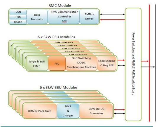
Possible system configurations with flexible redundancies 15kW N+1, 12kW N+2, 9kW N+3 or 9kW N+N
