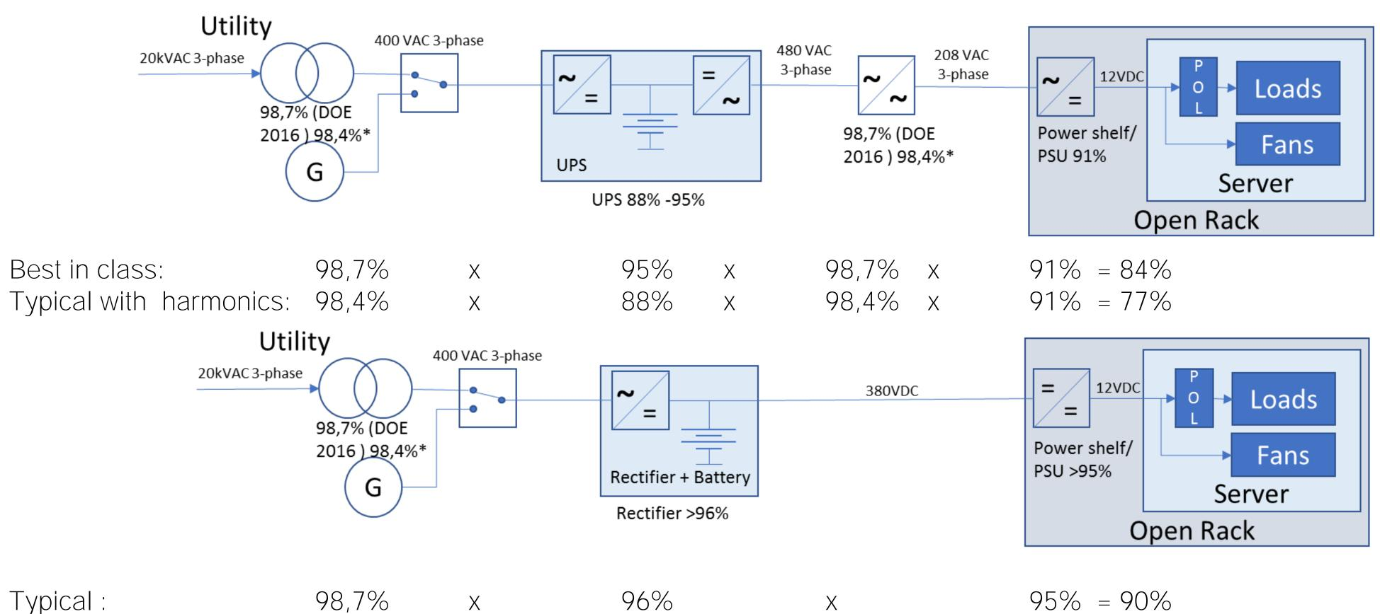
\*U.S. Department of Energy (US DOE) Limit. Transformer losses can increase 17% due the harmonics. Transformer losses in windings increase as the square of the THD, and that core losses increase linearly with the THD,
