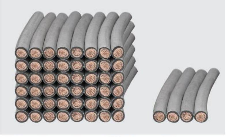
Figure 1. Cable required to transport 200 kW of current 245 feet with 48V DC compared to 400V DC. By courtesy of Vertiv
