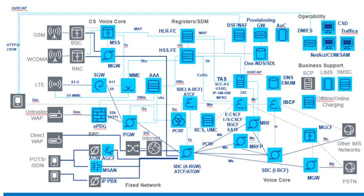
Network functions today run on purpose built bare metal hardware  $\rightarrow$  huge effort to operate and maintain networks where almost every box runs on a different platform.
