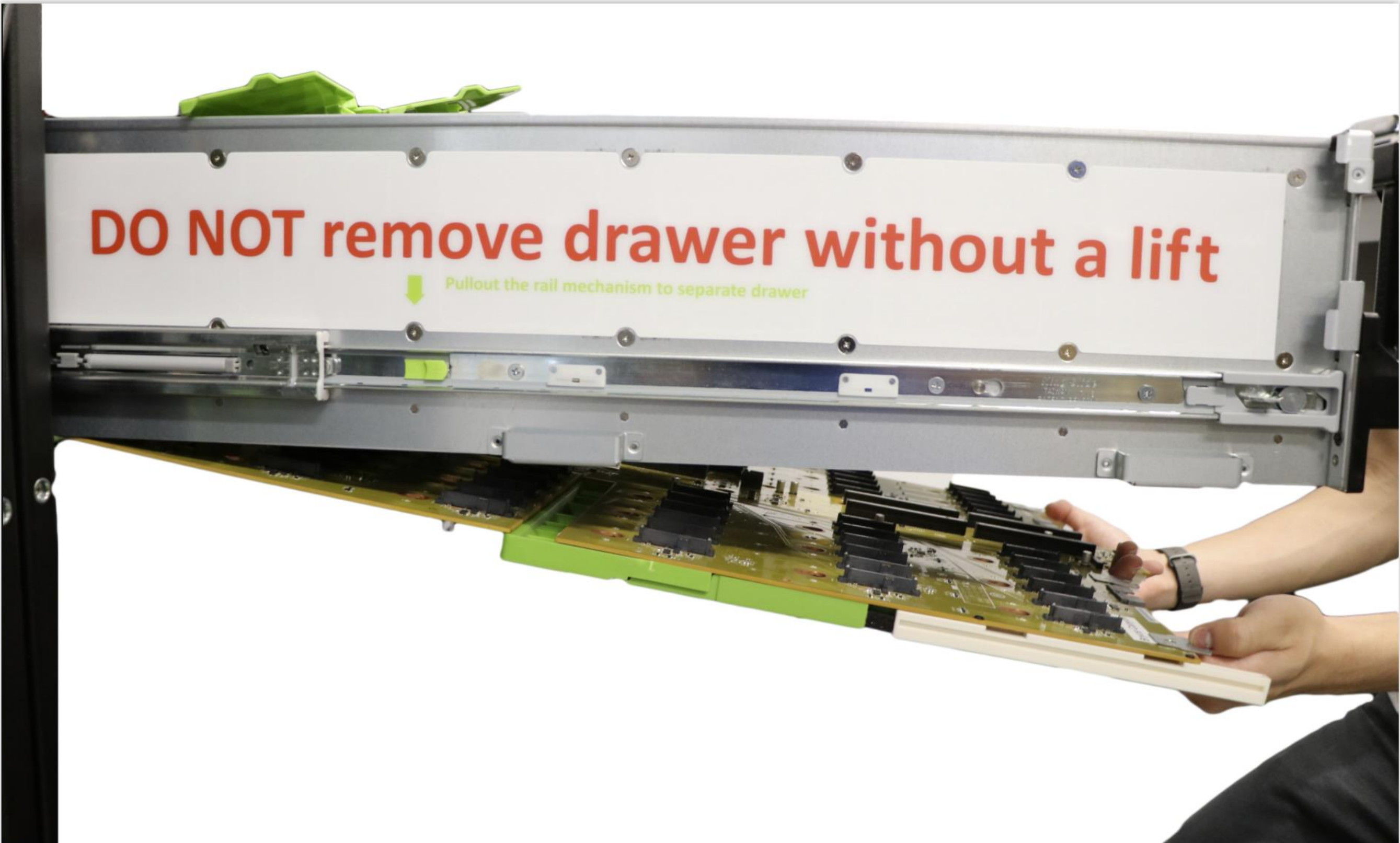
One piece backplane replacement
