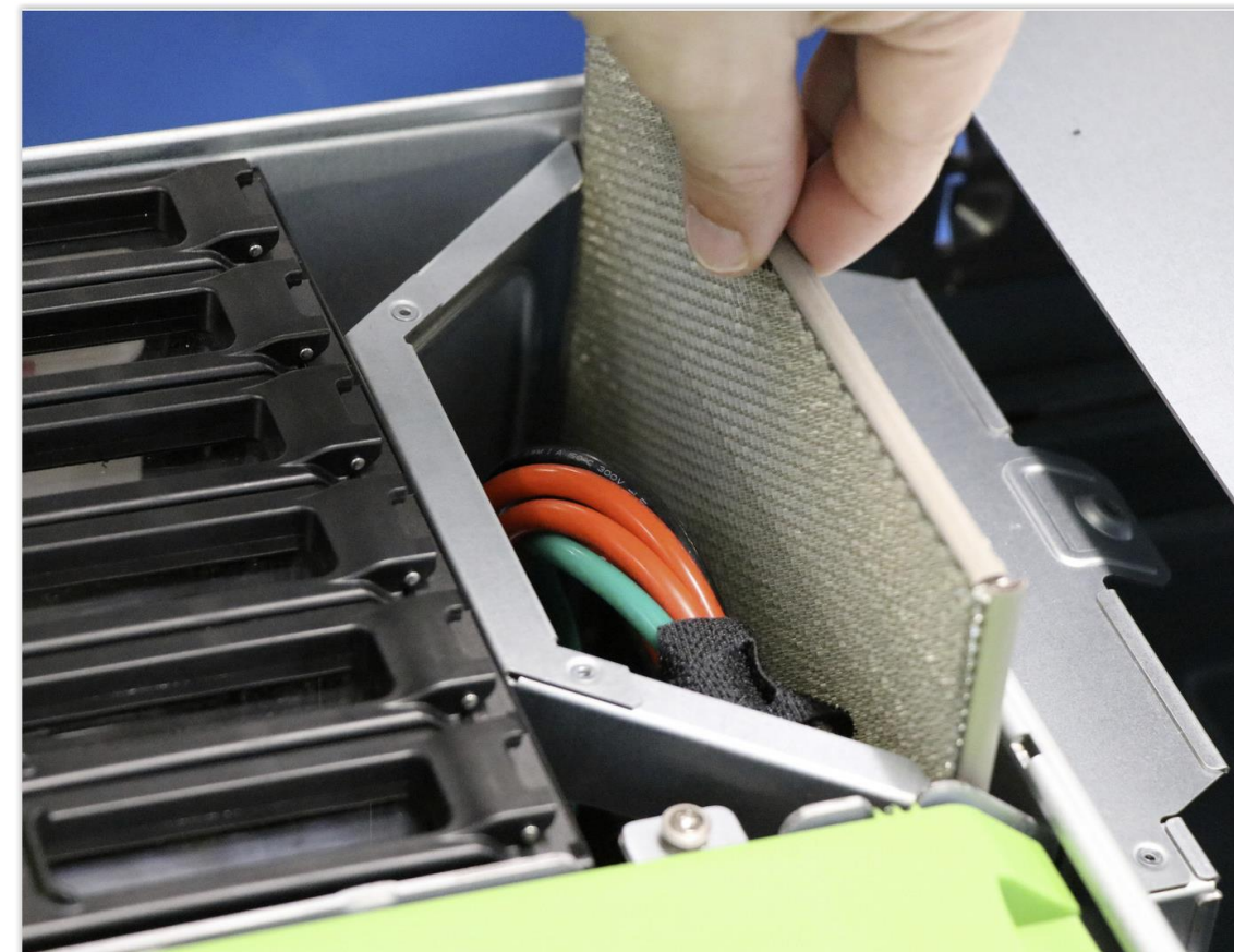
Honeycomb acts as acoustic attenuator
