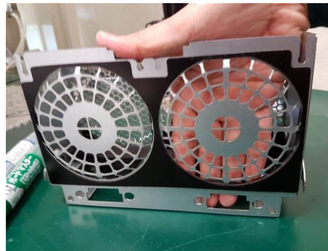
Smaller stamped metal vents
