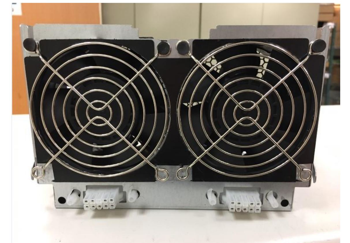
Larger wireframe guard vents
