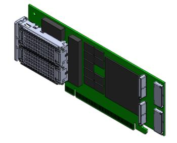
Xilinx ZU19P MPSoC FPGA +Xilinx ZU19P MPSoC FPGA +8x 2TByte M.2 NVMe SSDs +4x PCIe G4x8 cabled Storage IO50GB/s Dataplane Fabric IO50GB/s Dataplane Fabric IO
