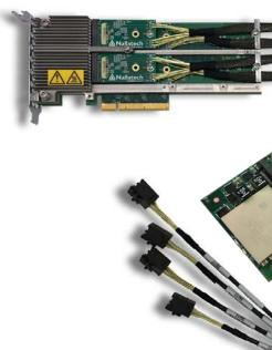
Altera 5SGXA7 FPGA to Fiber Channel Interface Xilinx KU060 FPGA + 2x 1TByte M.2 NVMe SSDs
