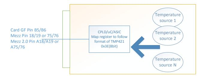
A register mapping of TMP422/TMP423 can be used to support one/two more temperatures in card implementation. The slave address of emulated device is always 0x3E, even it emulates TMP422/TMP423.
